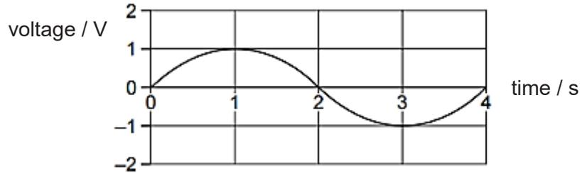
Some adjustments are made to the a.c. generator to produce the following graph.
