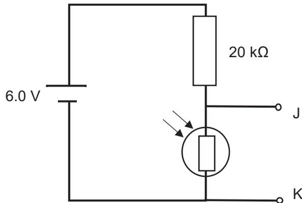
The resistance of the fixed resistor is  $20\text{ k}\Omega$ . The potential difference across JK is  $0.60\text{ V}$  when the lamp is switched on.
