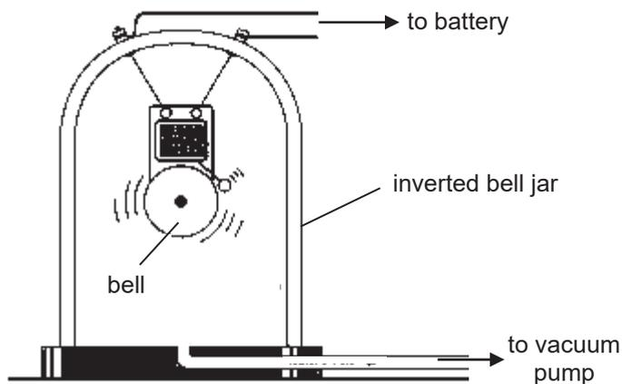
What happens to the pitch and loudness of the sound when the vacuum pump is switched on?
