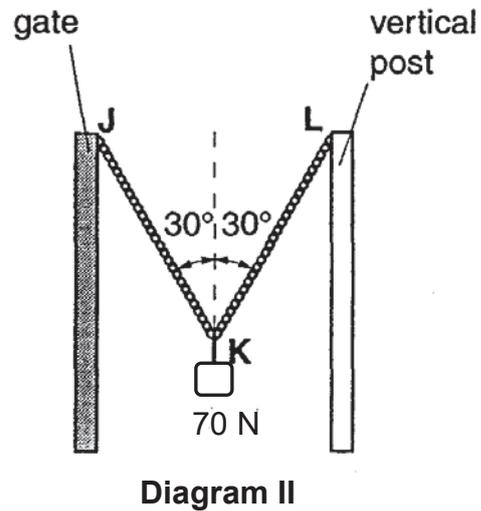
A heavy stone is attached by chains **JK** and **KL** to the top bar of the gate and to the top of a nearby vertical post. Opening the gate raises the stone. When the gate is released, the force exerted by the chains **JK** and **KL** closes the gate.
