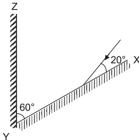
After reflection from XY, the ray is incident on YZ.
