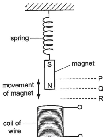
Where is the bottom of the magnet when there is no induced electromotive force in the coil?
