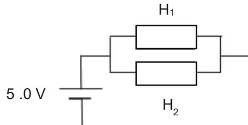
If  $P_1$  and  $P_2$  are the powers dissipated in heaters  $H_1$  and  $H_2$  respectively, which of the following is correct?
