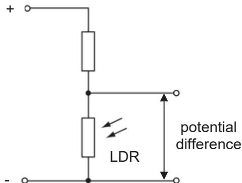
Which row shows the effect on the resistance of the light-dependent resistor (LDR) and on the potential difference (p.d.) across it as it gets brighter?
