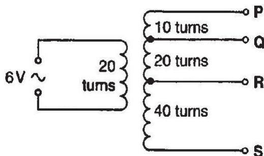
Between which two terminals will the output be 12 V?
