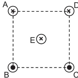
Which of the following **incorrectly** describes the resultant force on conductor E, with current flowing into the page, at the centre of the square?
