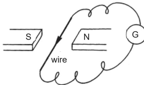
In which direction must the wire be moved to induce a current flow in the direction as shown in the diagram?
