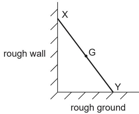
Its weight  $W$  acts through the centre of gravity  $G$ . Forces also act on the ladder at  $X$  and  $Y$ . These forces are  $X$  and  $Y$  respectively.
