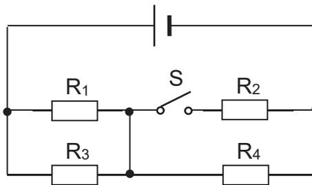
When switch  $S$  is opened, what are the powers dissipated in resistors  $R_3$  and  $R_4$ ?
