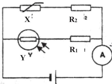
Which of the following changes to the electrical components  $X$  and  $Y$  will decrease the reading of the ammeter by the greatest amount?
