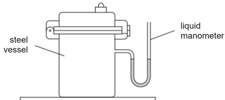
Which option describes the pressure in the vessel as indicated by the liquid manometer?
