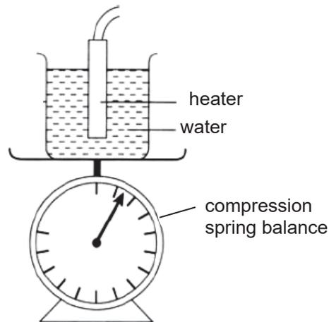
Three readings are taken by the compression spring balance.
