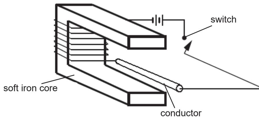
After the switch has been closed for a while, in which direction is the magnetic force acting on the conductor?
