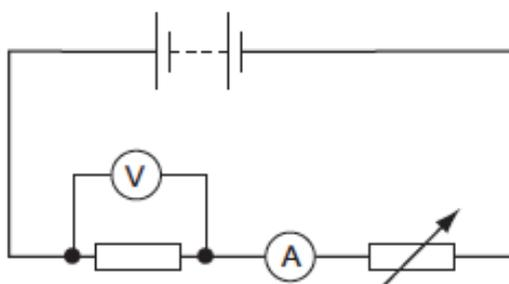
The resistance of the variable resistor is reduced.
