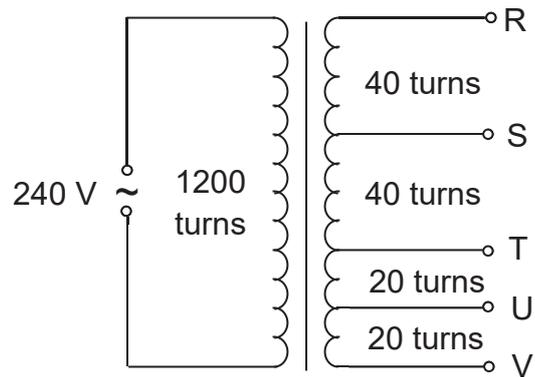
Which pair of terminals should be connected to a 12 V, 24 W lamp for it to be lit normally?
