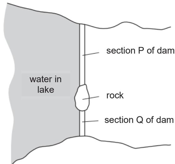
The water exerts a total force on each section of the dam and an average pressure on each section of the dam.
