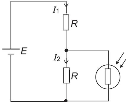
How do the currents change when the light intensity on the LDR is reduced to zero ?
