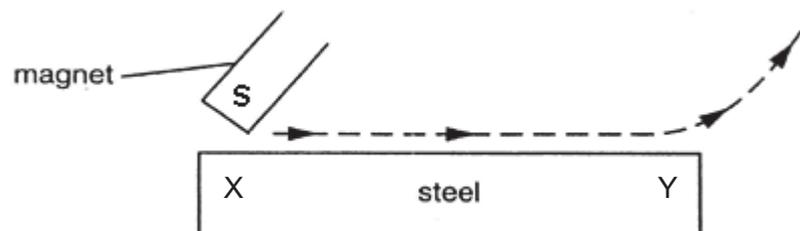
When the magnet is moved in the direction shown, which poles are produced at X and at Y?
