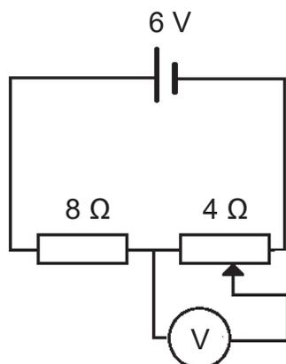
What are the minimum and maximum readings which can be obtained on the voltmeter?
