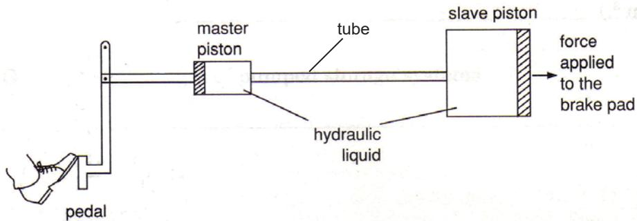
If the driver presses down on the pedal such that a force of 450 N is applied on the master piston, what is the force applied by the slave piston to the brake pad?
