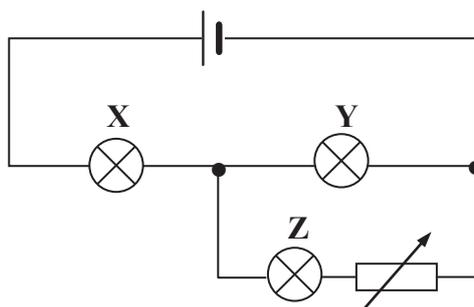
What will happen to the brightness of the lamps if the resistance of the rheostat is increased?
