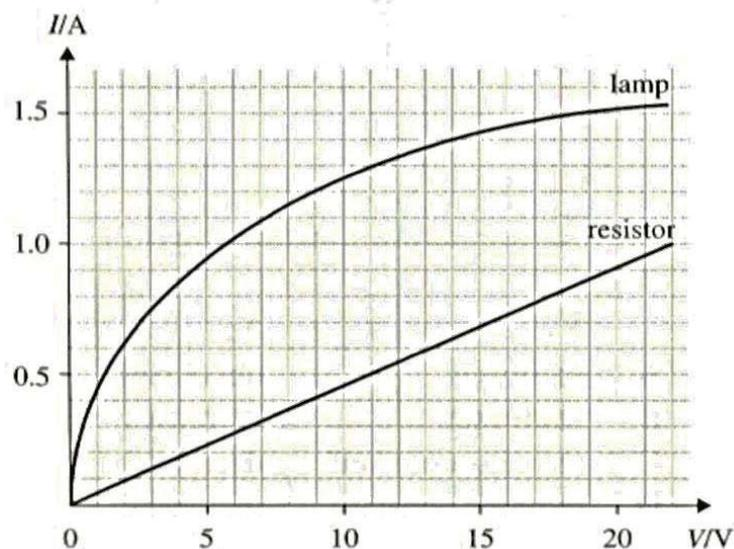
The lamp and the resistor are connected in series as shown below, and the ammeter reading is 0.6 A.
