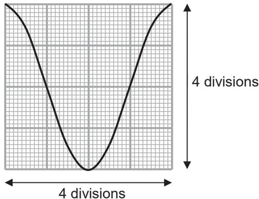
The time-base is set to 2.0 ms/div and the voltage sensitivity is 2.0 V/div. Which of the following correctly represents the peak voltage and frequency of the signal?
