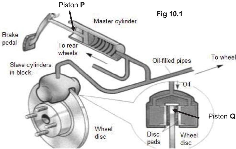
A force is applied downwards on the brake pedal in order to slow down the wheels of the car.
