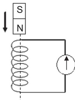
How does the galvanometer needle move as the magnet falls away from the coil?
