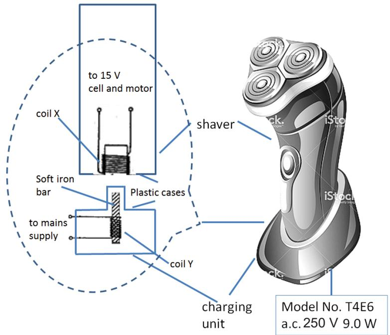
It consists of the shaver and a charging unit. Both the shaver and the charging unit are completely covered by plastic cases and there is no metal contact between them. Inside the shaver, there is a 15 V rechargeable cell for driving a motor.
