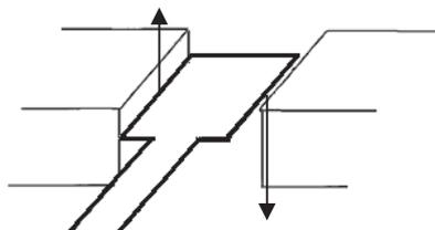
**11(b)** The coil rotates in a clockwise direction about its axis [A1] for about a maximum of  $90^\circ$ . As the current is not reversed at this juncture, the coil continues to stay in the vertical position. [A1]
