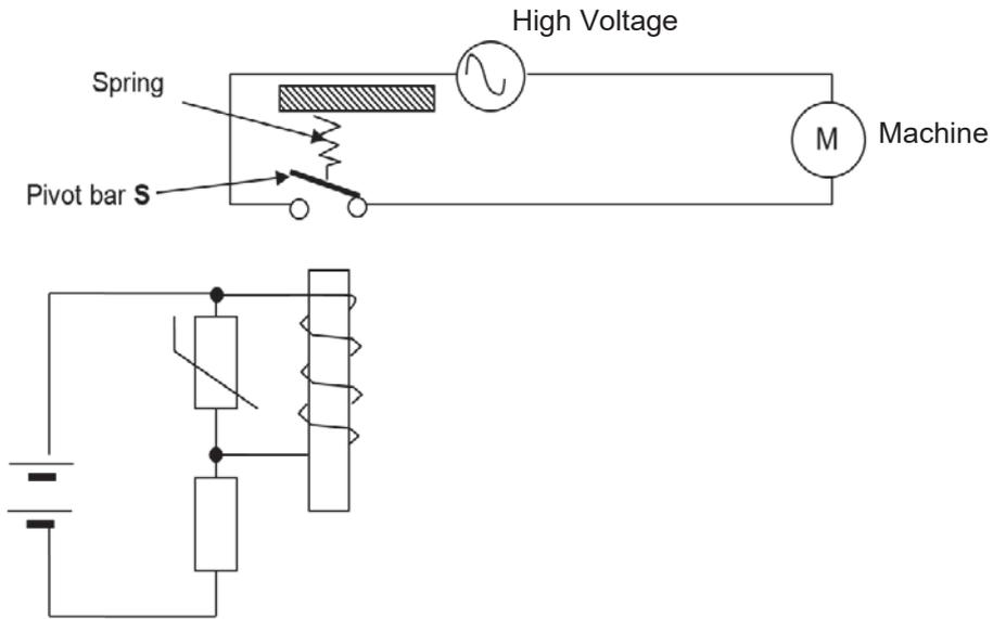
(a) Explain how the magnetic relay works when the temperature around the thermistor **decreases**.
