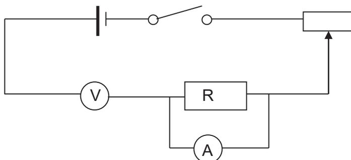
What are the readings on the ammeter A and voltmeter V when the jockey is adjusted to give minimum resistance and the switch is closed?
