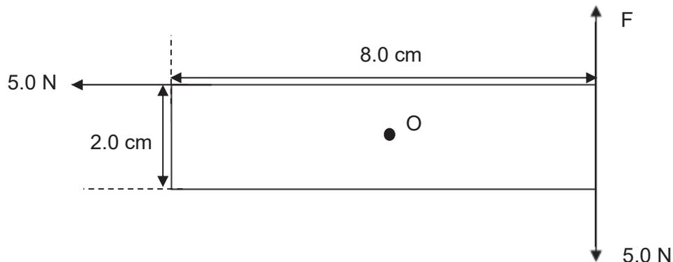
What is the size of force F such that the cardboard does not rotate about pivot O?
