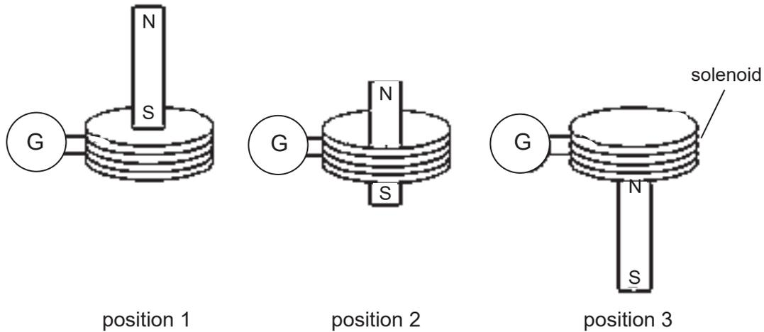
At which position(s) will the galvanometer show a deflection?
