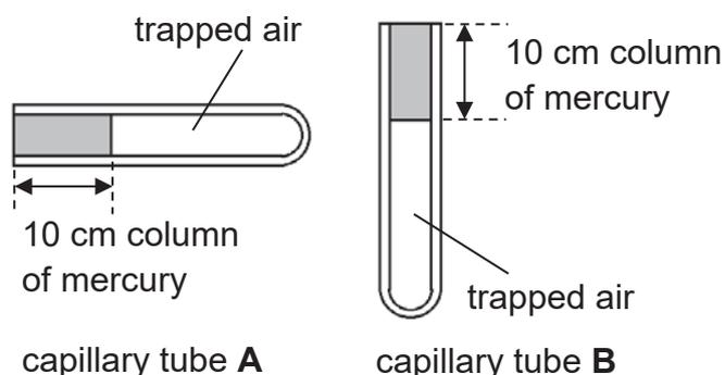
What is the pressure of the trapped air in capillary tubes **A** and **B**?
