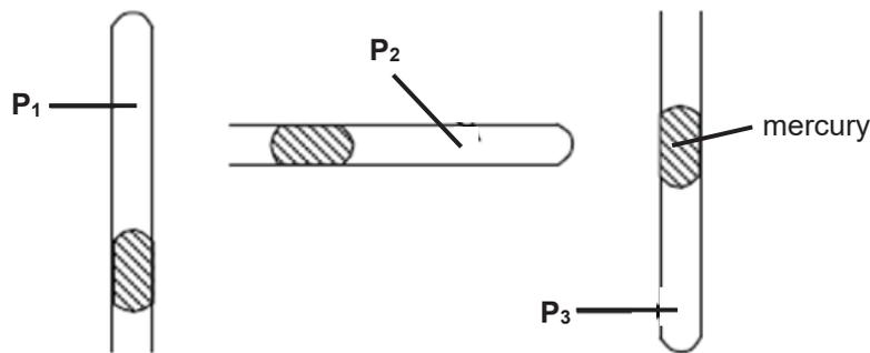
$P_1$ ,  $P_2$  and  $P_3$  are pressures of the enclosed air in the capillary tube. Which relationship is correct?
