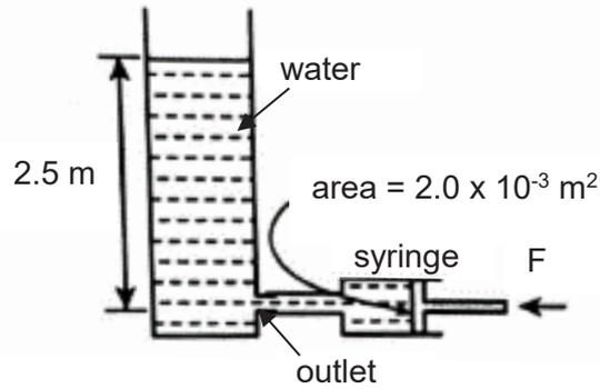
What is the minimum force  $F$  that must be applied to the piston of the syringe to prevent it from moving outwards?
