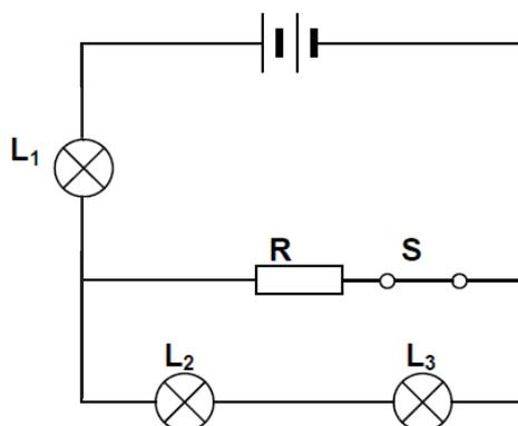
How will the brightness of lamps  $L_1$ ,  $L_2$  and  $L_3$  change when the switch  $S$  is opened?
