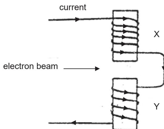
In which direction will the electron beam be deflected?
