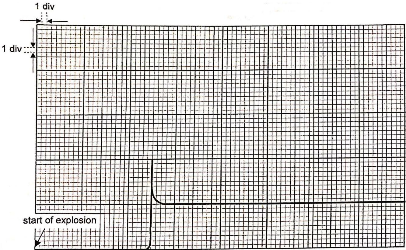
The amount of light is measured in lux. Given that the y-gain scale is 50,000 lux/div and time base scale is 120 ns/div,
