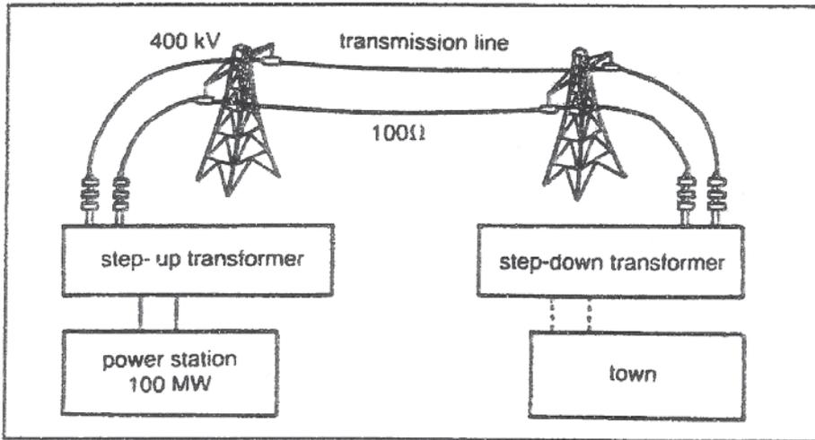
The voltage is stepped up to 400 kV and the national grid transmits the power over a large distance. The voltage is then stepped down before the power is used by industries and homes in a town.
