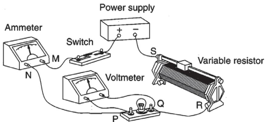
Which one of the following shows the correct circuit diagram?
